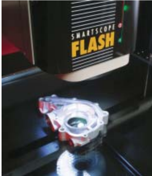
A video measurement of a cast metal part is illuminated by an LED ringlight. Photo: Optical Gaging Products
