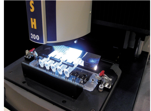
A multi-part fixture with fold mirror for measuring all the dimensions of several plastic syringe bodies in a single setup.
