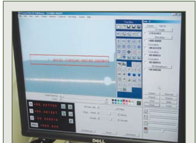
▲ To ensure the staged part is correctly oriented, the optical gage performs an auto-alignment. This is represented by a red rectangle on the screen. Also, note the 0.0050-inch through-hole.
