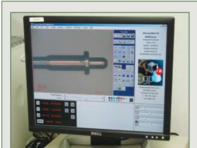
▲ The magnified display for the Smart Scope helps the operator identify obvious errors on the part as well as burrs. On this barrel part, 55 measurement steps are performed in 20 seconds.
