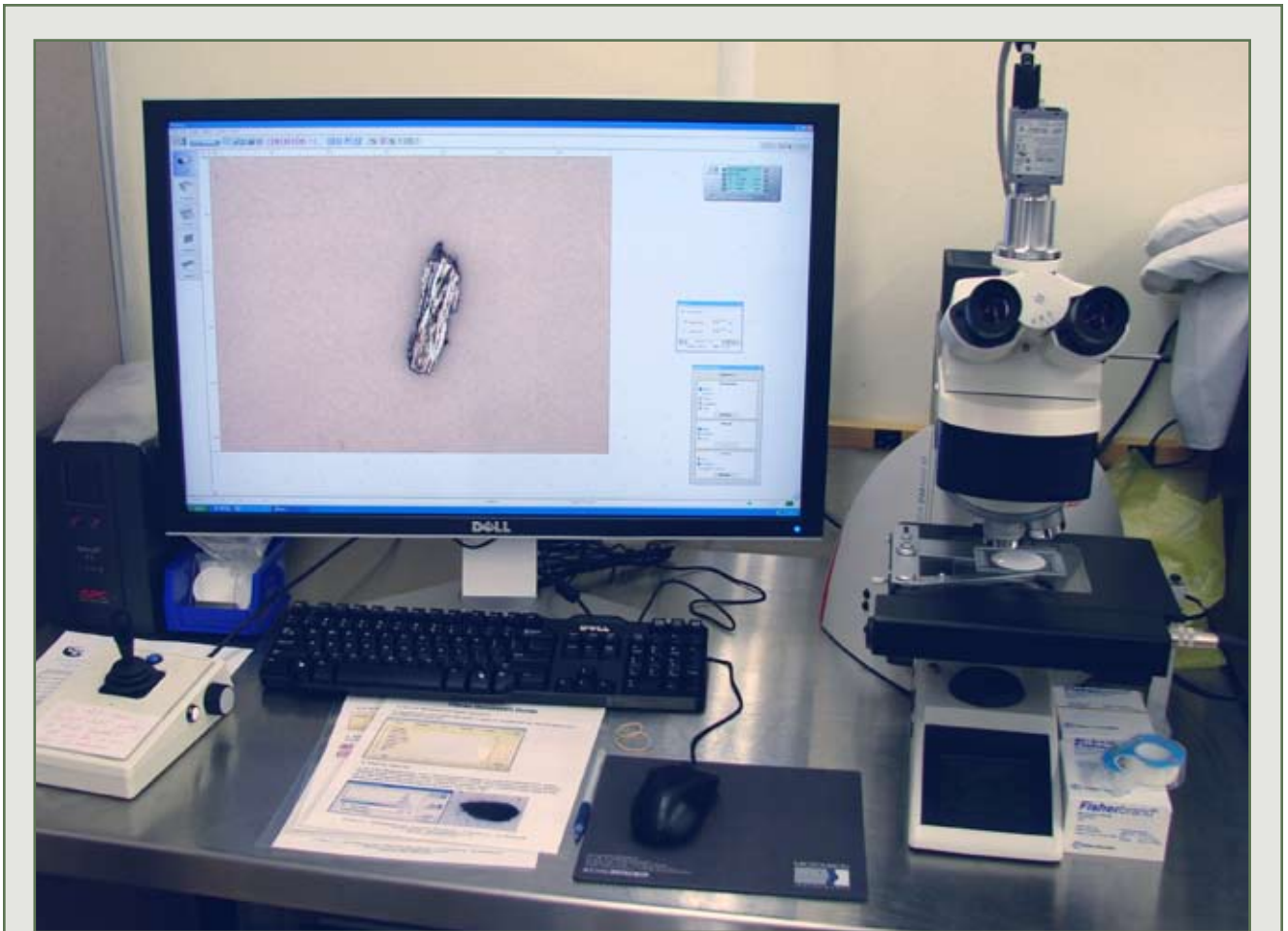
▲ American Micro's particle counting microscope does double duty for cleanliness specifications and high res magnification for part inspection. The image on the screen is a particle that measures roughly 150 × 70 microns.
