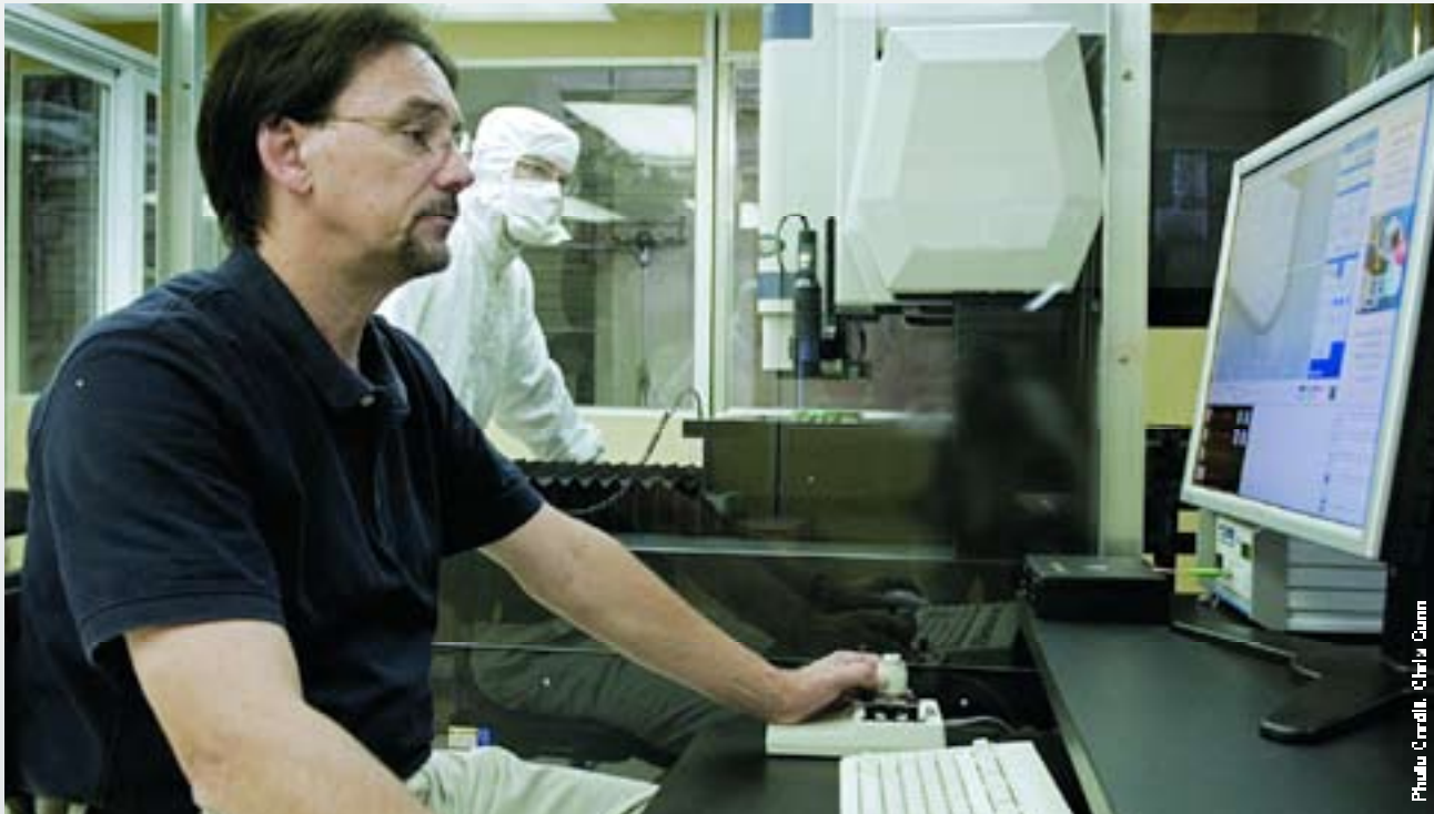
The Smartscope is the latest addition to Goddard's Advanced Manufacturing Branch. A highly precise measurement tool, it is now housed in a Class-100 clean room in Building 5. George Bertholdt (in the forefront) operates the machine.
