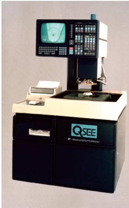
**Circa 1985, this system has a membrane touch panel, HP Thinkjet printer and dual 3½ inch floppy disk drives. Source: Optical Gaging Products Inc.**
