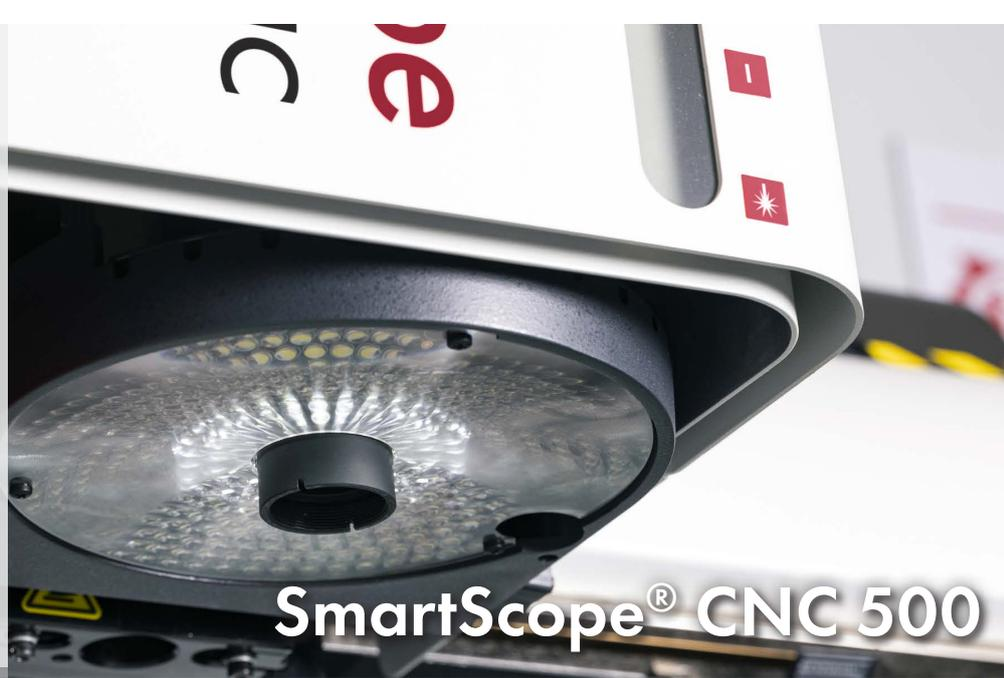
**SmartScope CNC 500** – Offers all the great CNC features and performance in a large travel fixed bridge design. Parts move on a precision DC motor-driven Y-axis stage while the optics assembly travels in the X-axis across a stable bridge cross member. Optics mounted on a rigid bridge support structure for metrological integrity. CNC 500 provides:
