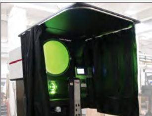
Light Curtain controls excess ambient light.
