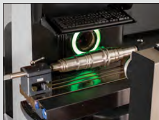
Extended Travel – standard stage travel can be extended up to 18 inches on both c-vision models
