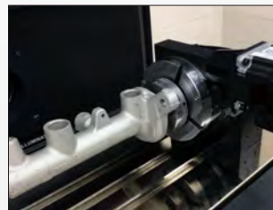
Programmable Motorized Rotary Indexer for staging shafts and cylinders.
