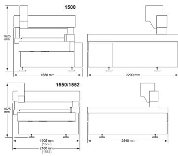
Flash 1500 System Weight: 2590 kg Shipping Weight: 3000 kg Flash 1550 System Weight: 5460 kg Shipping Weight: 6260 kg Flash 1552 System Weight: 6380 kg Shipping Weight: 7280 kg
