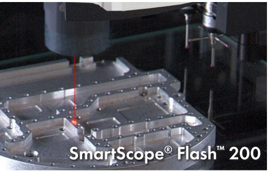
SmartScope Flash 200 – One of the most popular 3D multisensor dimensional measurement systems on the market. The elevating bridge provides a larger working area than similar designs. Flash 200 offers:
