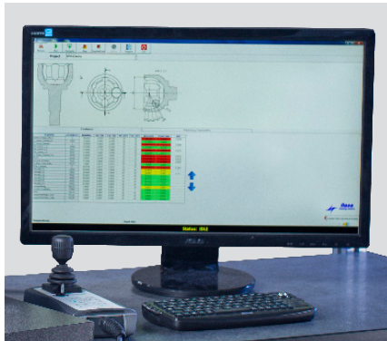
Tangram metrology software performs dimensional calculations on critical part information.
