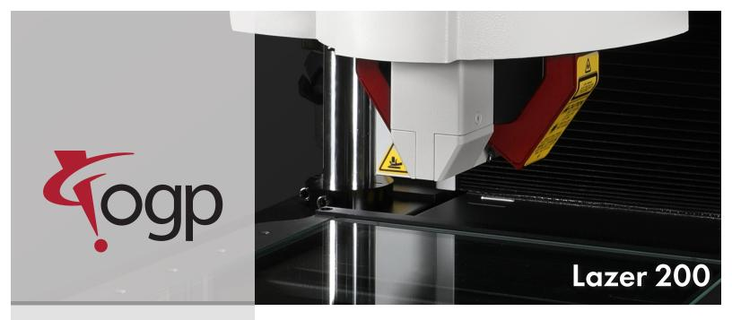
Lazer 200 – An innovative noncontact measuring system that uses laser scanning for surface topography measurements. The Digital Range Sensor (DRS™) laser delivers high quality non-contact laser scans of critical part surfaces. Lazer 200 features:
