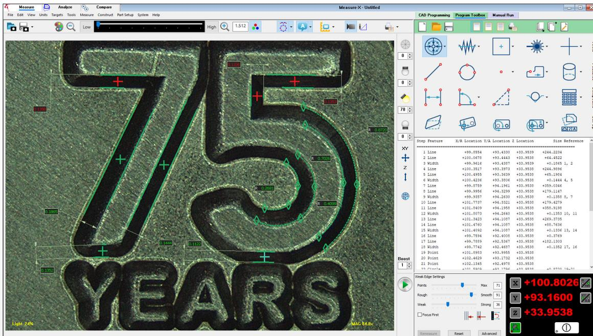
From creating part measurement routines to operating an OGP® system in a production work environment, **Measure-X®** metrology software offers power without intimidation. Measure-X features a full set of image processing and autofocus tools, geometric functions, ANSI/ISO tolerances, easy editing, and contour fitting analysis. Measure-X is the ideal choice for general-purpose video and multisensor metrology.
