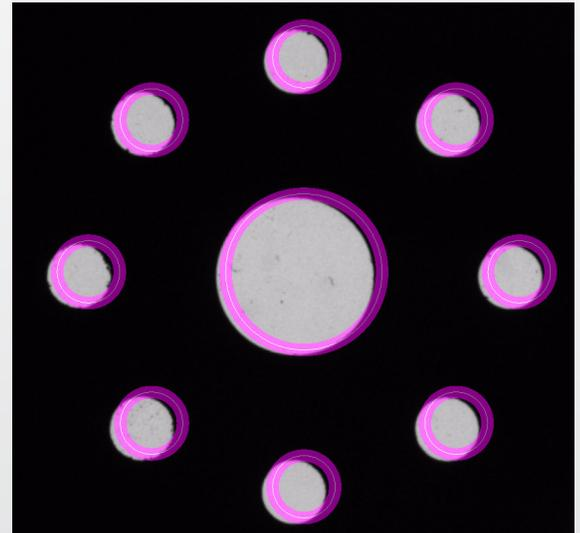
In **Analyze** mode, GD&T results can be viewed to easily visualize the results based on fitting of data acquired in Measure mode. Feature control frame flyouts, along with color-coded whiskers and tolerance bands, are shown to provide a graphical representation of the analysis. The direction of the whiskers allows operators to easily determine whether there is excess or lack of material.
