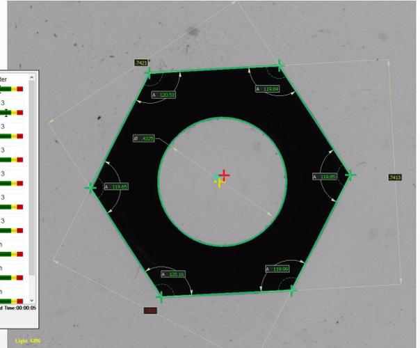
In **Compare** mode, operators can visually inspect results relative to overlay charts for direct comparison of the actual part to the nominal dimensions using a live video image. This “virtual chart gage” is as large as the part, and can extend beyond the viewing area, independent of magnification.
