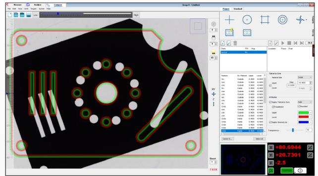
**VidiProbe** transforms the traditional optical comparator into a fully automatic video inspection system using Measure-X software. An internal video camera is positioned to view the image formed by the comparator optics, allowing the image to be digitally analyzed and measured instantly using automatic edge detection.
