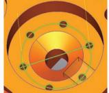
**Constructions** of bolt hole circle and maximum distance between two holes in that circle.
