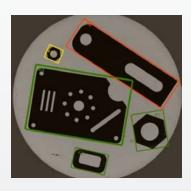
Use **AutoID** to automatically run a routine. ZONE3 will search for and automatically run part routines that match the part(s) that you have placed on the machine stage and are visible within the video window.
