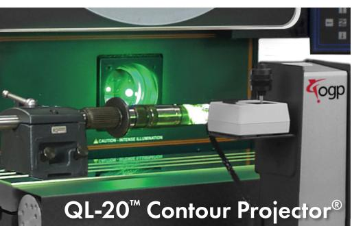
The **QL-20** optical comparator is a precision instrument designed for the shop floor. QL-20 has extensive standard features and a range of options that allow you to configure a system to meet your specific measurement needs.
