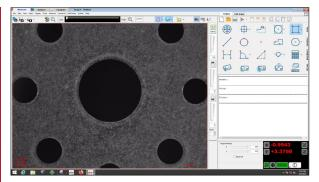
Transform the traditional optical comparator into a fully automatic inspection system with optional VidiProbe and Measure-X® software. The video camera is internally mounted to enable simultaneous measurements using both the analog comparator screen and the digital video with Measure-X.
