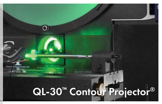
The **QL-30** is an ultra-high capacity optical comparator that offers a large, bright image and compact footprint.
