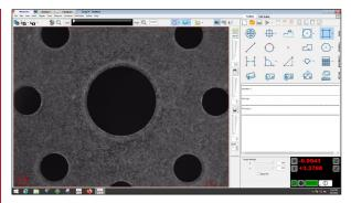
Transform the traditional optical comparator into a fully automatic inspection system with optional VidiProbe and Measure-X<sup>®</sup> software. The video camera is internally mounted to enable simultaneous measurements using both the analog comparator screen and the digital video with Measure-X.
