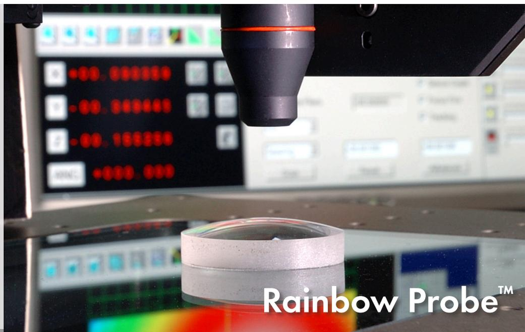
**Rainbow Probe** is a non-contact chromatic confocal sensor that measures surfaces by analyzing changes in the optical spectrum as a function of part to probe spacing. Additional capabilities include:
