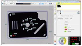
SNAP-X software provides users with a simple, powerful interface for instant 2D measurement and auto program generation. The software also utilizes powerful GD&T based algorithms and point and click feature identification to easily program a wide variety of parts. Virtual chart gaging, profile analysis tools and integrated reporting allow for quick and easy output of measurements.
