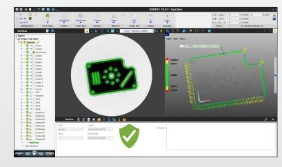
**ZONE3 Express** offers full measurement capabilities and tools, basic GD&T functionality, and the ability to work with 2D CAD files.
