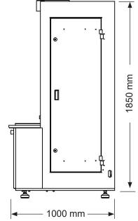
Machine Weight: 350 kg Crated Weight: 450 kg
