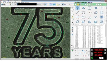
Full feature Measure-X® metrology software offers 2D CAD program generation and general-purpose dimensional measurement with multisensor and rotary axis support.
