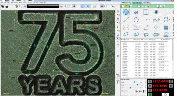
Full feature Measure-X® metrology software offers 2D CAD program generation and general-purpose dimensional measurement with multisensor and rotary axis support.
