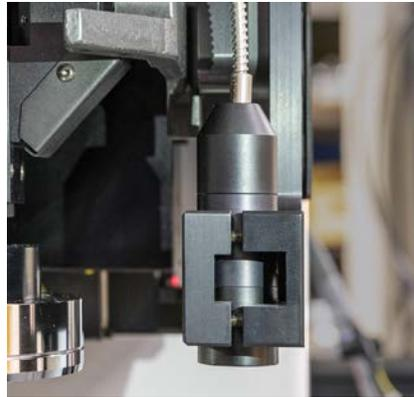
P-25-70 integrated on a SmartScope ZIP with fixed mount
