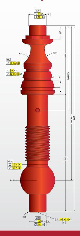
**TurnCheck** software is fast and easy to program with a focus on what you want to measure rather than how to measure it. Automatic feature extraction immediately finds and measures all part features in a single scan. A single image displaying the entire part allows you to easily see all basic shaft measurements at once. Rotational scans can be done for form and runout measurements providing plots to truly visualize the results.
