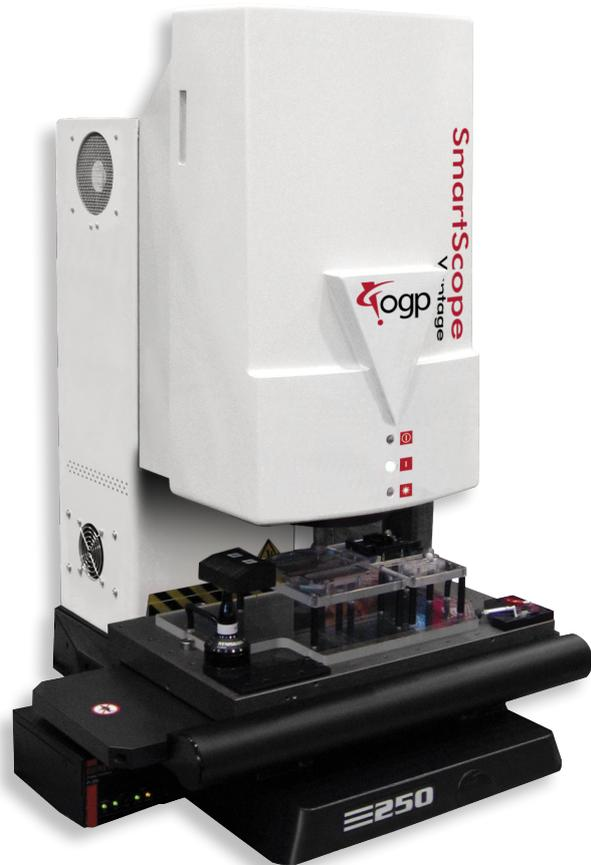
Equipped with optional touch probe and change rack.
