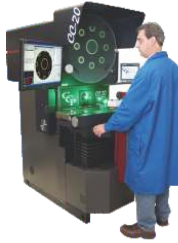
Actual image of virtual chart and part profile on a CCP comparator screen.
